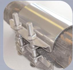
This mini clamp is as plain repair clamp. Suitable for repairing holes in small pipelines. The inside of the clamp is partially covered with a NBR or EPDM gasket. This design requires no welding and therefore no chemical treatment to passivate the clamps. Only available in predefined quantities of 100 units per position.
